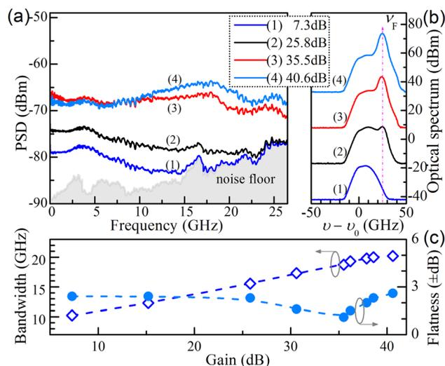
FIG. 3. Experimentally obtained effects of gain: (a) the power spectral density of the resonator outputs generated with different gains of 7.3, 25.8, 35.5, and 40.6 dB at detuning of 25 GHz, (b) the corresponding optical spectra, and (c) the bandwidth ( $\diamond$ ) and spectral flatness ( $\bullet$ ) as the functions of gain.
