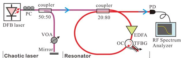
FIG. 1. Experimental setup. The resonator consists of a fiber ring equipped with an EDFA and a tunable fiber Bragg grating (TFBG). A DFB laser diode with external-cavity feedback from a mirror is used as the chaotic injection source. The spectral property of chaotic signal is measured by a RF spectrum analyzer. PC: polarization controller; VOA: variable optical attenuator; OC: optical circulator; PD: photodetector.
