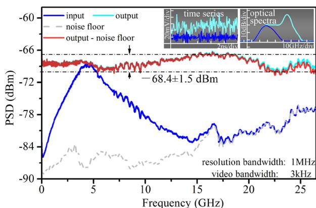
FIG. 2. Experimental improvement of PSD: the black (blue) and the gray (cyan) curves represent the chaotic laser and the fiber ring resonator output, respectively. The dark gray (red) curve is the output spectrum after subtraction of electronic noise (dashed line) of the RF spectrum analyzer. The insets plot the corresponding time series and optical spectra.
