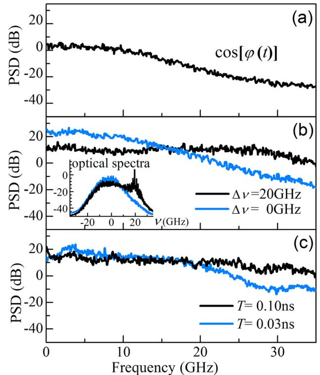
FIG. 5. Numerical PSD: (a)  $\cos\varphi$  of chaotic laser; (b) outputs at  $\Delta\nu = 20$  GHz (black) and  $\Delta\nu = 0$  GHz (gray, azure),  $T = 5 \text{ ns}$ , and the inset plots the corresponding optical spectra; (c) outputs at  $T = 0.1$  (black) and  $T = 0.03 \text{ ns}$  (gray, azure),  $\Delta\nu = 20$  GHz.
