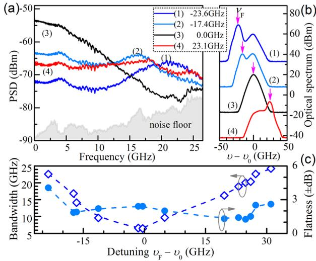
FIG. 4. Experimentally obtained effects of filter detuning: (a) the power spectral density of the resonator outputs generated at different detuning of  $-23.6$ ,  $-17.4$ ,  $0$ , and  $23.1$  GHz with intra-ring loss of  $-4.9$  dB, (b) the corresponding optical spectra, and (c) the bandwidth ( $\diamond$ ) and spectral flatness ( $\bullet$ ) as the functions of filter detuning.
