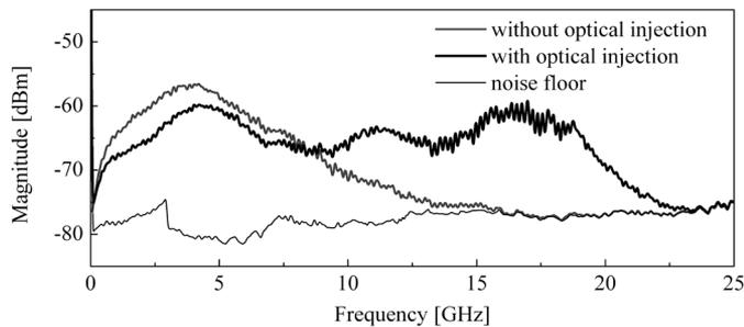
Fig. 2. Experimentally obtained spectrum of the bandwidth-enhanced chaotic signal (black bold line) with  $-5.6$ -dBm optical injection at  $8.8$ -GHz detuning. The gray thin line denotes the spectrum of original state of the chaotic laser without optical injection. The bandwidth is enhanced from  $6.2$  to  $16.8$  GHz. (Resolution bandwidth =  $3$  MHz).
