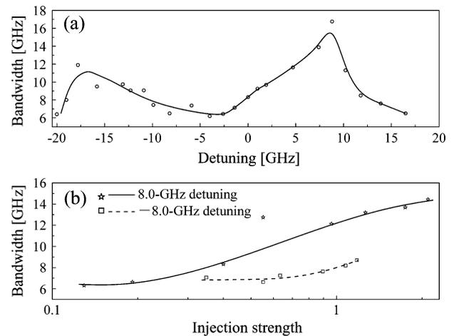
Fig. 3. (a) Experimentally enhanced bandwidths as a function of the detuning of  $-5.6$ -dBm injection light plotted with circles and fitted curve. (b) Bandwidths as a function of the injection strength at  $8.0$ -GHz and  $-8.0$ -GHz detuning depicted with stars and squares, respectively. The solid line and the dashed line are their respective regression curves.
