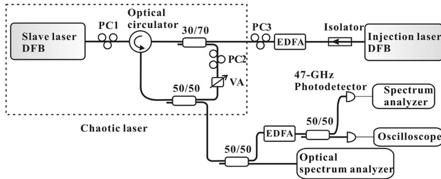
Fig. 1. Experimental setup of bandwidth enhancement of optical chaotic signal generated by chaotic laser with optical feedback using optical injection.
