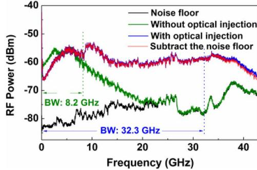
Fig. 2. Experimentally obtained spectrum of the broadband chaotic laser signal with  $-2.11$ -dBm injection power at  $25.4$ - and  $32.9$ -GHz detuning. The bandwidth is enhanced from  $8.2$  to  $32.3$  GHz. (Resolution bandwidth:  $1$  MHz; video bandwidth:  $1$  kHz.)
