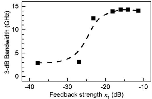
Fig. 5. Experimental bandwidth of the heterodyne signal as a function of feedback strength  $\kappa_1$ , obtained with  $\kappa_2 = -19.5$  dB and  $\nu_{c2} - \nu_{c1} = 12.5$  GHz.
