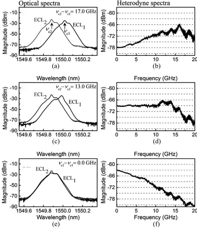
Fig. 6. (a), (c), and (e) Optical spectra of ECL<sub>1</sub> (black) and ECL<sub>2</sub> (gray) and (b), (d), and (f) RF spectra of the heterodyne signals experimentally obtained at different detuning of lasers frequencies: (a) and (b) 17.0 GHz, (c) and (d) 13.0 GHz, and (e) and (f) 0 GHz. The feedback strength  $\kappa_1 = -15.9$  dB,  $\kappa_2 = -19.5$  dB.
