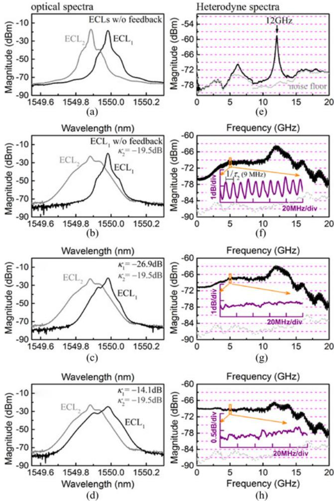
Fig. 4. (a)–(d) Experimental optical spectra of ECL<sub>1</sub> (black) and ECL<sub>2</sub> (gray) and (e)–(h) RF spectrum of the corresponding heterodyne signal: (a), (e) ECLs are both without feedback, (b), (f) ECL<sub>1</sub> without feedback,  $\kappa_2 = -19.5$  dB, (c), (g)  $\kappa_1 = -26.9$  dB,  $\kappa_2 = -19.5$  dB, and (d), (h)  $\kappa_1 = -14.1$  dB,  $\kappa_2 = -19.5$  dB. The detuning of laser center frequencies is 12.5 GHz.
