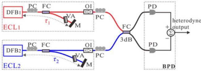
Fig. 1. Experimental setup of white chaos generation using the optical heterodyning of two external-cavity feedback lasers (ECLs). Each ECL consists of a DFB semiconductor laser with optical feedback from a fiber mirror (M).  $\tau_1, \tau_2$  are the round-trip time in feedback cavities. PC: polarization controller; FC: fiber coupler; VA: variable attenuator; OI: optical isolator; PD: photodetector; BPD: balanced photodetector.
