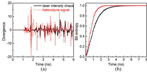
Fig. 11. (a) Divergence of two temporal waveforms numerically generated at the same initial conditions when different noise sequences are added at  $t = 0$ ; (b) Bit entropy as a function of time. Gray (red online), the heterodyne signal; black, laser chaos.
