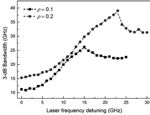
Fig. 9. Numerically obtained bandwidth of the heterodyne signal as a function of detuning of lasers' frequencies, obtained with  $\rho_{1,2} = 0.10$  (squares) and  $\rho_{1,2} = 0.20$  (circles), respectively.
